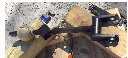
The photo at left shows the bell arriving with yoke and clapper attached. Both needed to be taken off the bell for it to fit into the tower. Photos at right show the new yoke and clapper.
