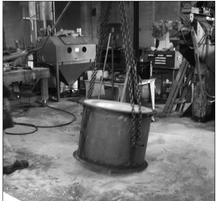
Figure 10. Drag lifted and inverted to expose inside of bell.
