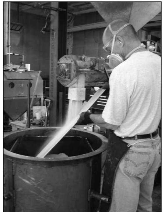
Figure 6. Metal bar deflects silica sand into the flask.
