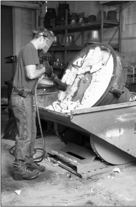
Figure 45. Chiseling out the inner profile of the mold material.
