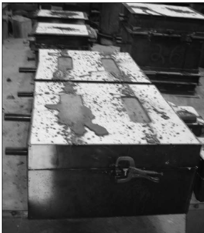
Figure 43. Smaller bell molds poured.
