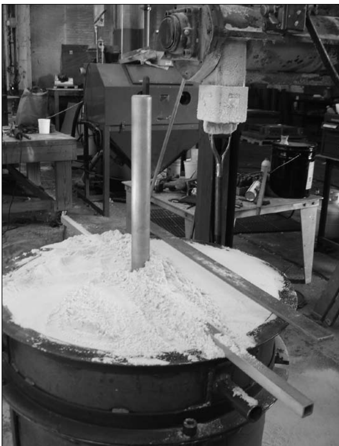
Figure 16. Cope/drag filled and leveling begins.
