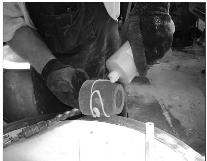
Figure 27. Ceramic material with glue applied to outside.
