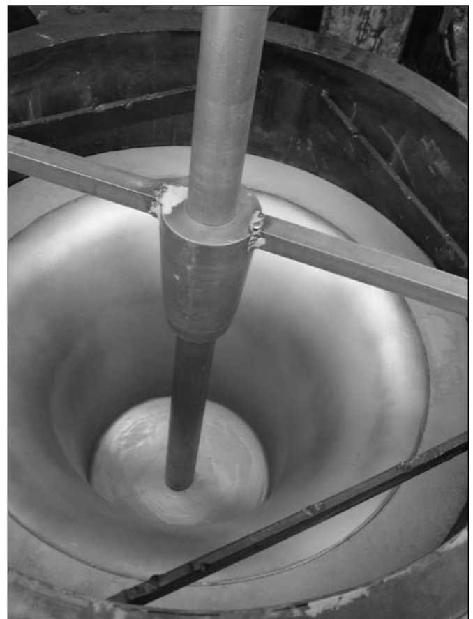
Figure 14. Gate added to the inside of the bell pattern.
