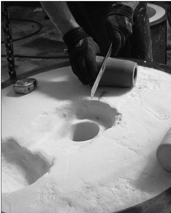
Figure 24. Ceramic material cone being cut to proper dimensions.
