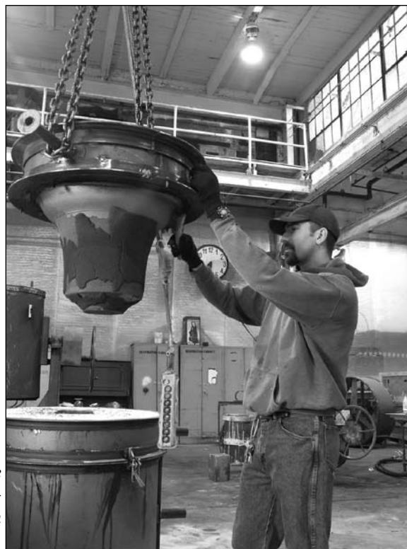
Figure 44. Cope and drag separated by Tim Verdin.
