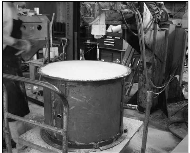
Figure 9. Leveled flask waiting to cure.
