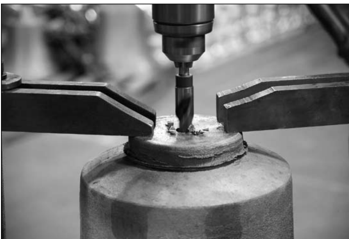
Figure 47. Hole drilled for hanging the bell.
