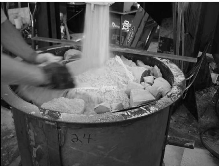
Figure 8. Chunks of previously used material placed on the outer edges of the flask.
