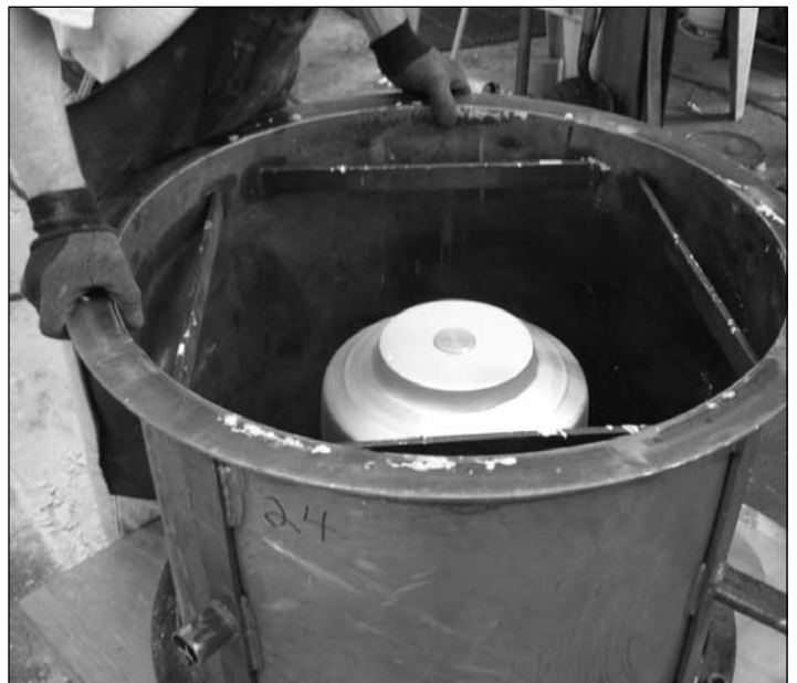
Figure 2. Inside view of bell pattern inside drag flask.
