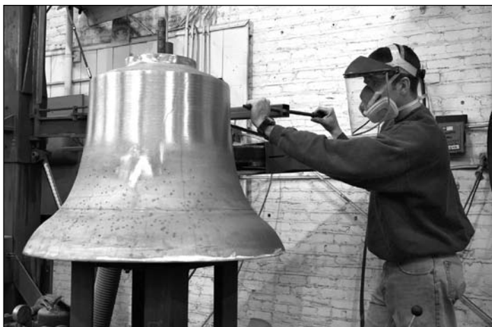
Figure 52. Close-up of one of the stages in the polishing of the bell.
