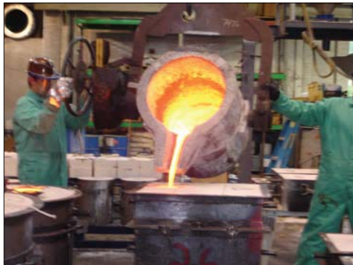
Figure 40. Twenty-six inch bell being poured.
