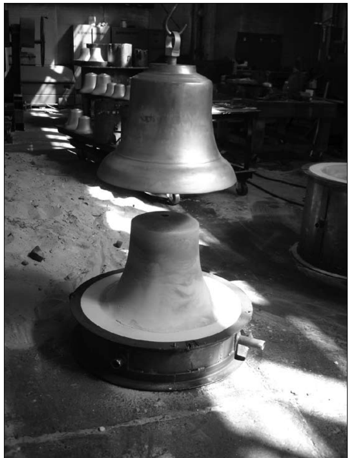
Figure 22. Bell pattern being removed from bell mold.
