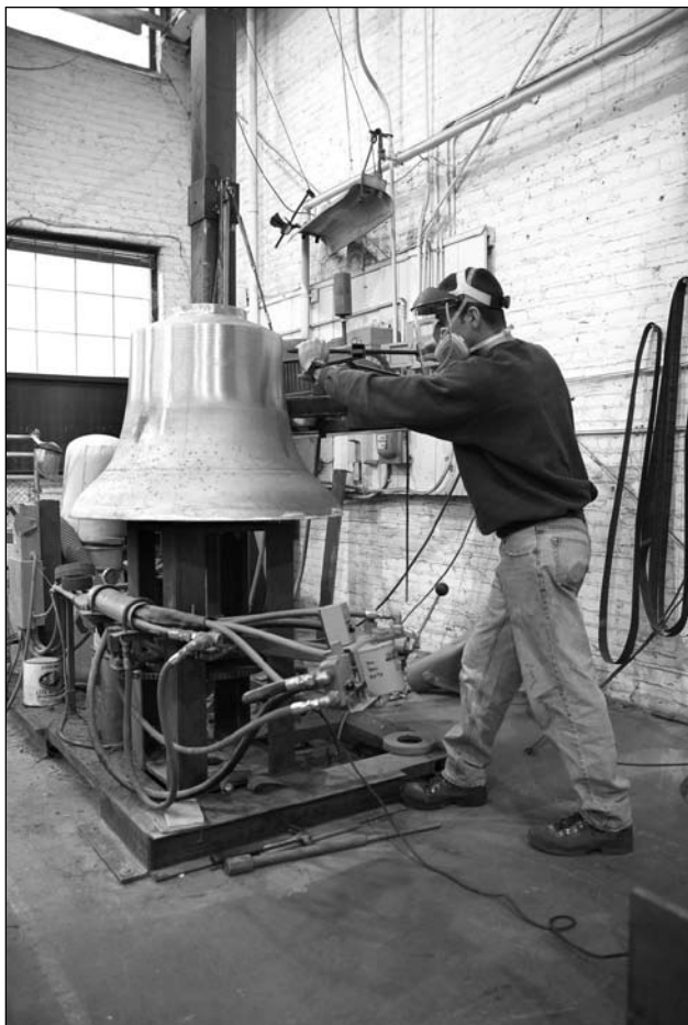
Figure 51. Custom polishing of bell.
