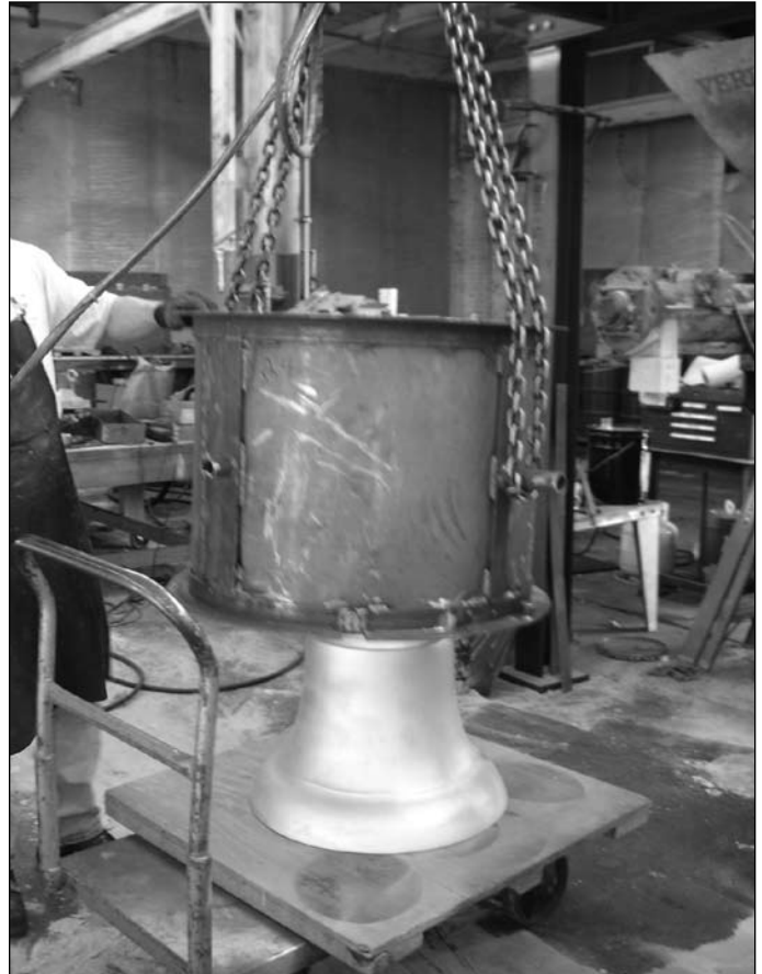
Figure 1. Bell pattern on bottom board; drag flask lowered over bell pattern.
