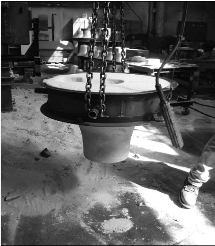
Figure 23. Cope section being inverted.
