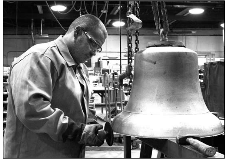
Figure 48. Dean Issacs removes extra metal from the pour.
