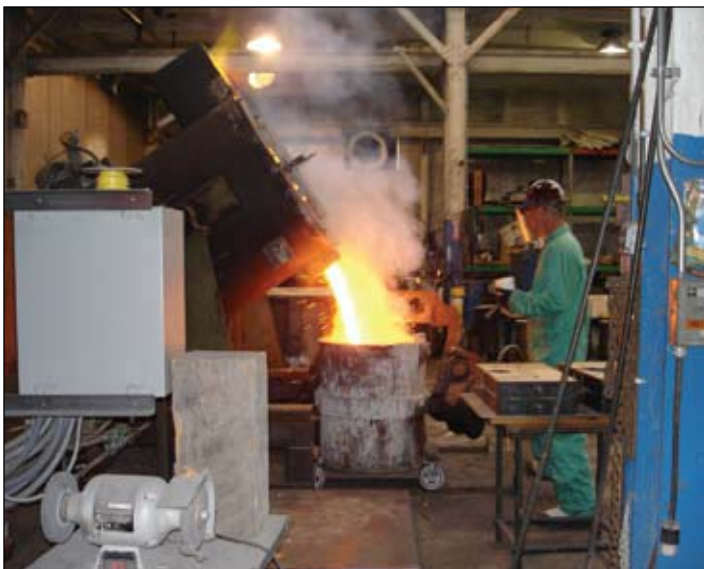
Figure 38. Ralph adds flux to the large ladle.
