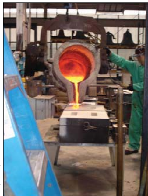
Figure 42. Smaller 12" bells being poured from the large ladle.
