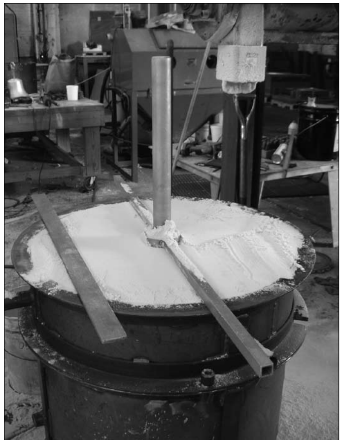
Figure 17. Cope leveled while the sand mixture begins to set up.
