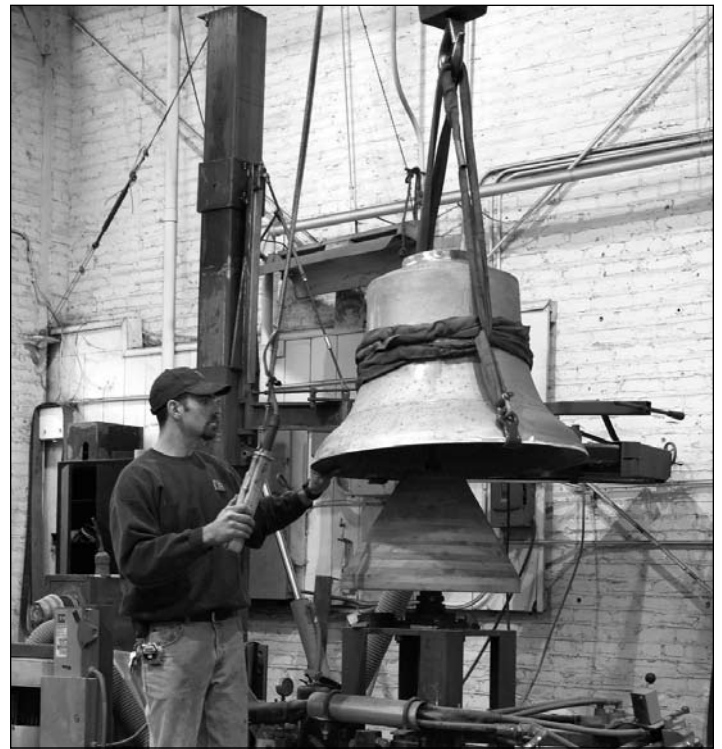
Figure 49. Tim Verdin places bell on a custom polishing machine.
