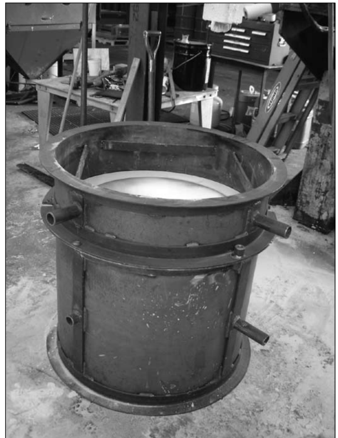
Figure 13. Cope section added to the drag section.
