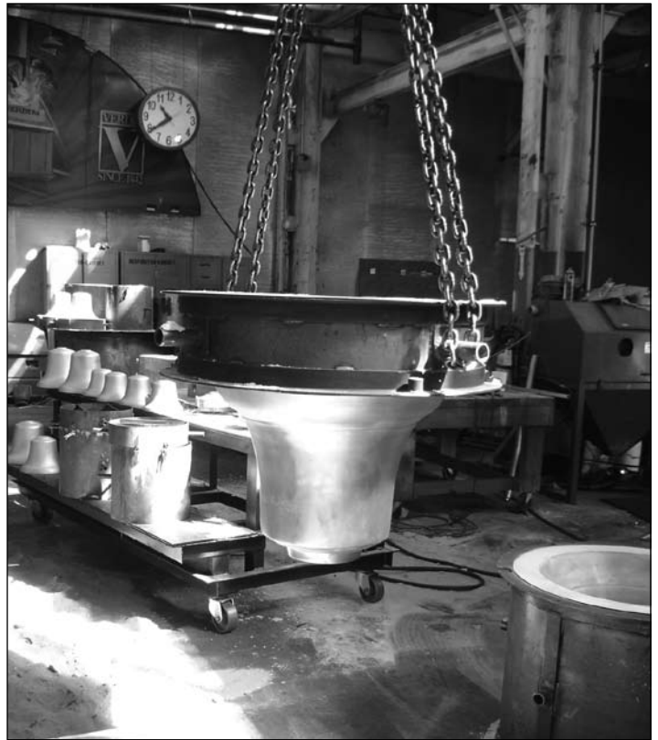
Figure 21. Cope being removed from flask.
