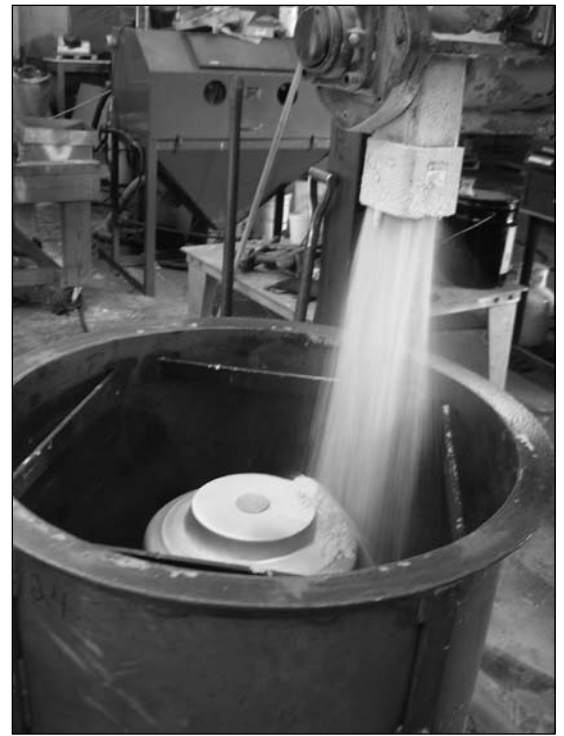
Figure 5. Silica sand added to the drag flask.
