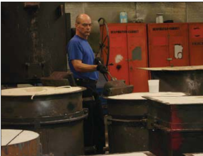
Figure 32. Ralph heats the ingot molds.
