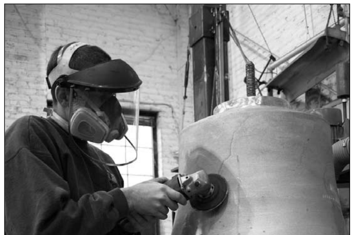
Figure 50. Polishing begins on the bell.
