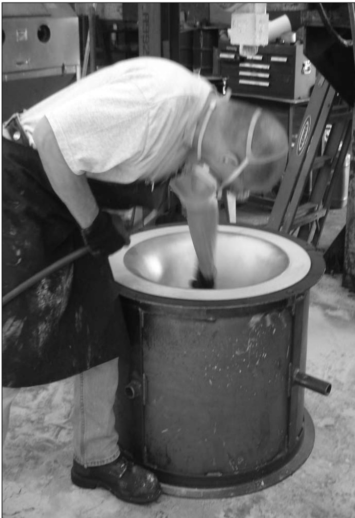
Figure 12. Inside of bell being air pressured to remove any dirt particles.
