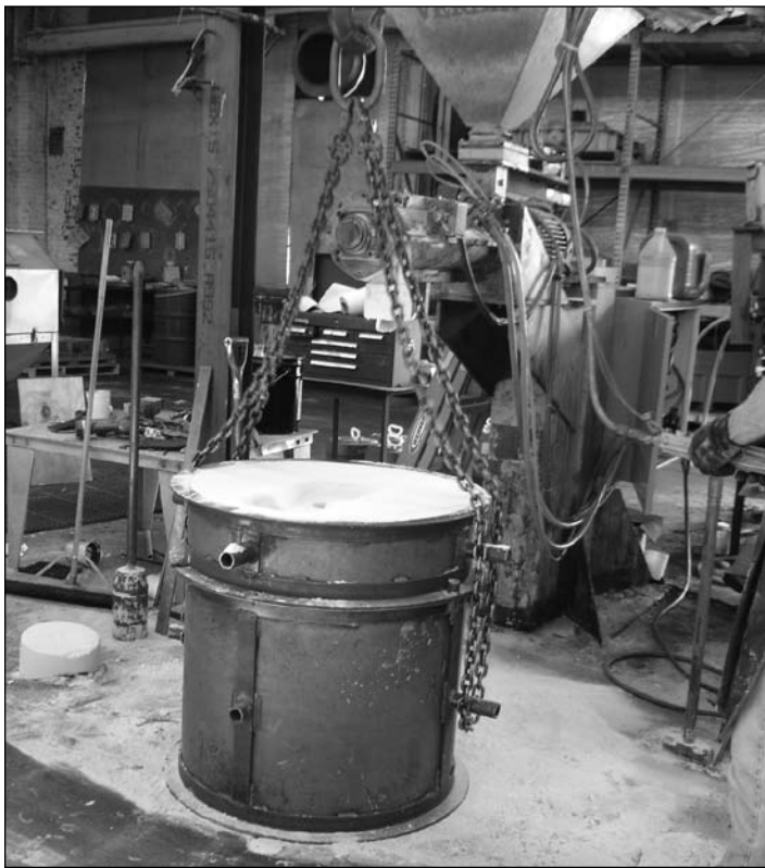
Figure 20. Completed mold with pattern in place (flask).
