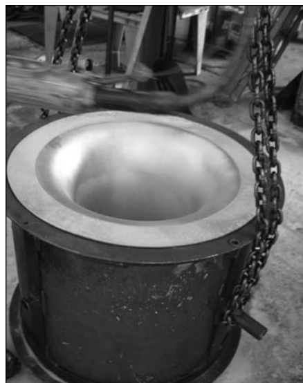
Figure 10. Drag lifted and inverted to expose inside of bell.
