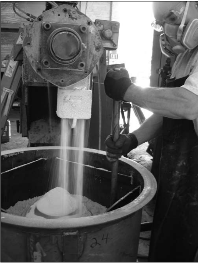
Figure 7. Another inside view of the flask filling.
