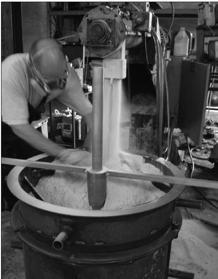
Figure 15. Inside of bell filling with silica sand.
