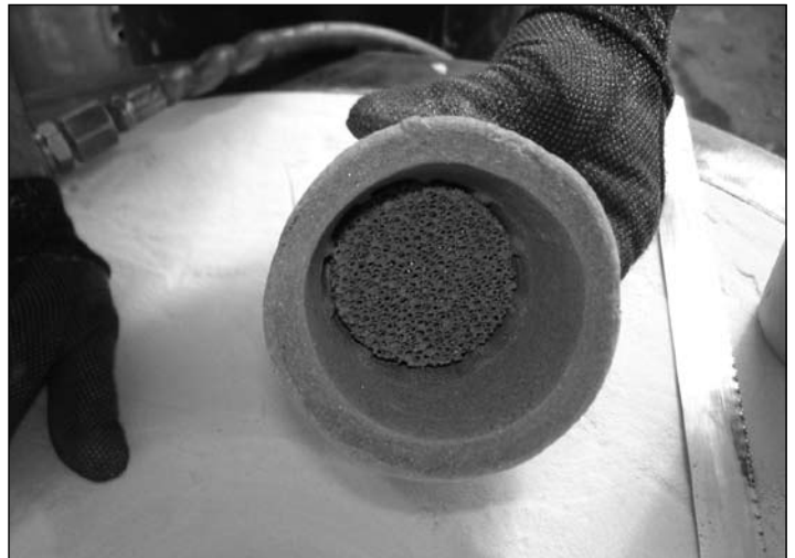
Figure 26. Filter placed into the ceramic cone.
