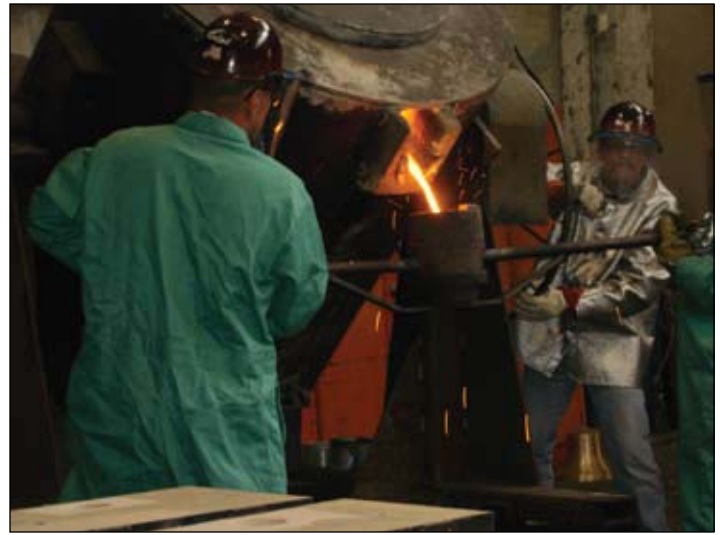
Figure 34. Tommy Robinson angles furnace pour spout to the exact location; Ralph and Tommy gather the molten bronze into the ladle.
