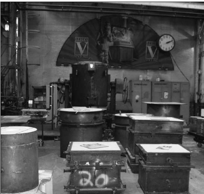
Figure 29. Various bell molds prepared for pouring.
