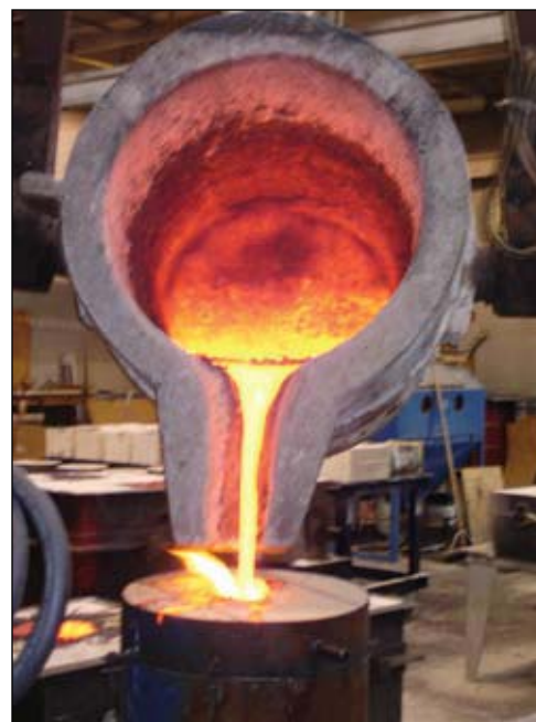
Figure 41. Close-up view of the molten bronze with flame shooting from the sprue hole.
