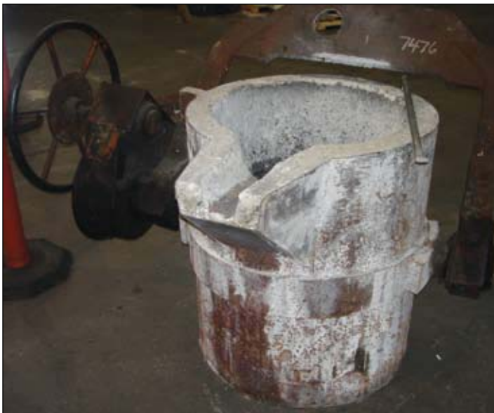
Figure 37. Larger ladle that will be used to pour the 20", 24", and 26" bells.
