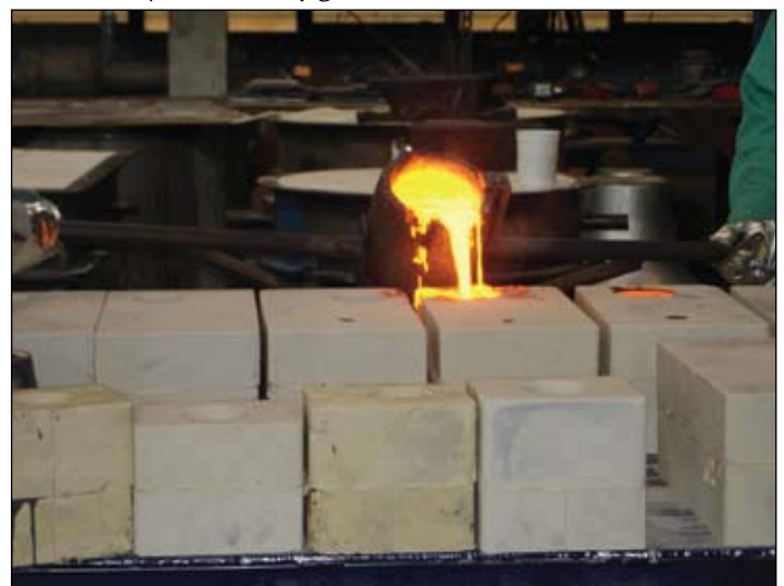
Figure 35. Various size bells being poured from the ladle.
